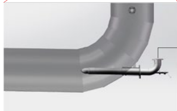
Stock Injector installed in the Approach Flow piping
